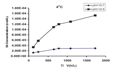
Fig. 3a. Silicon concentration (mol/l) as a function of the time profile (DT/DV) at 4 °C
