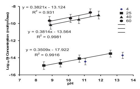
Fig. 4. Rate of stilbite dissolution at variable temperatures and in situ pH based on Si release
