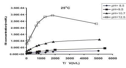
Fig. 3b. Silicon concentration (mol/l) as a function of the time profile (DT/DV) at 25 °C
