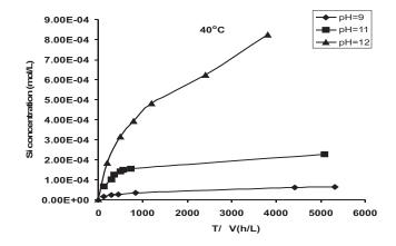
Fig. 3c. Silicon concentration (mol/l) as a function of the time profile (DT/DV) at 40 °C
