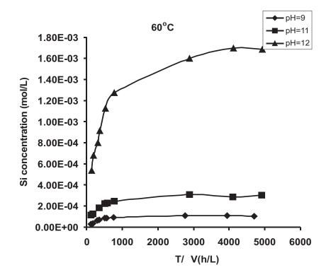
Fig. 3d. Silicon concentration (mol/l) as a function of the time profile (DT/DV) at 60  $^\circ \rm C$
