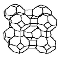
Fig. 2. Structural matrix of a zeolite
