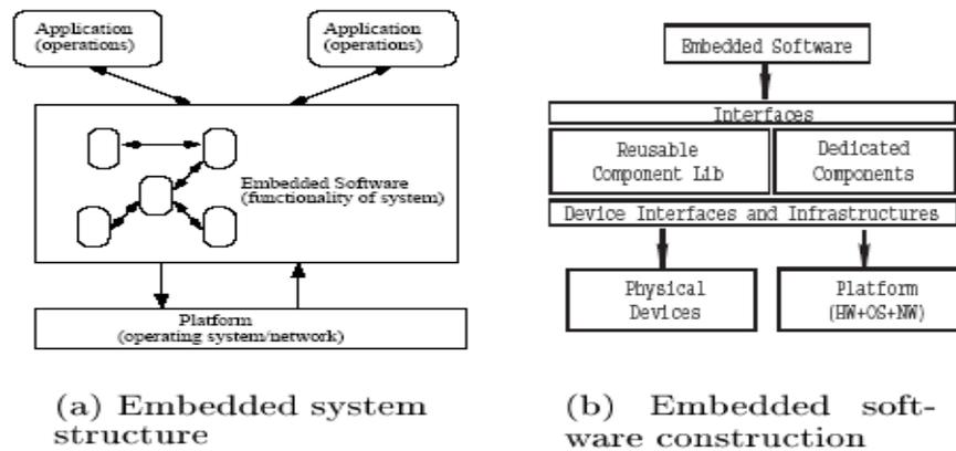
**Fig. 4: Integration of embedded software**
