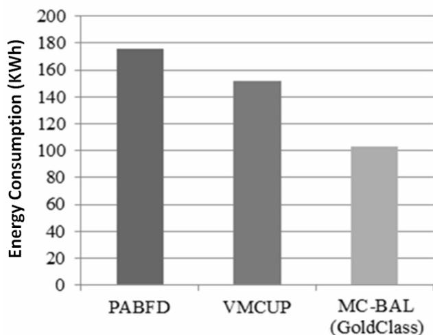
Fig. 1. Comparison of Total Energy Consumption - PlanetLab dataset
