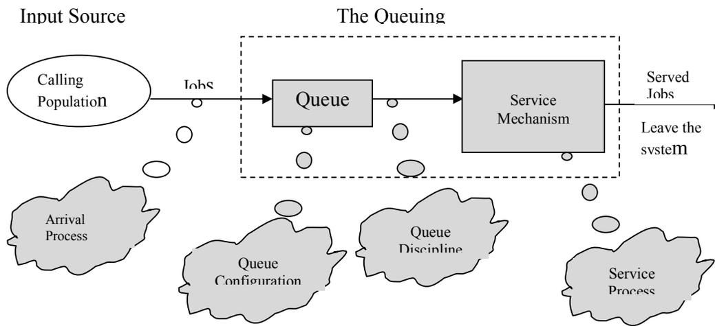
**Fig. 2.1: Components of a queuing system**
