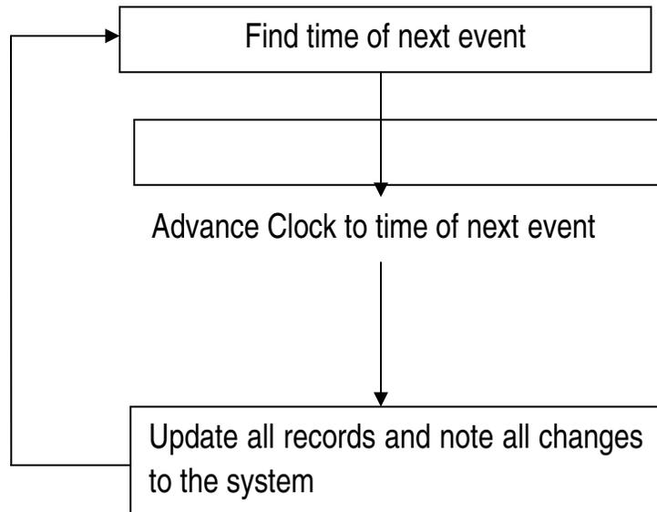
**Fig. 3: Algorithm Design Summary Flow Diagram**
