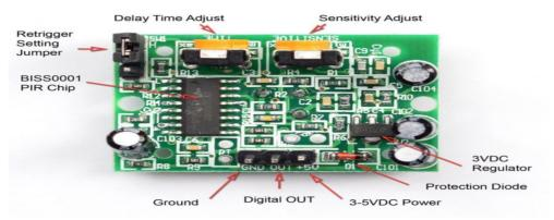
Figure 2: PIR module's upper view. (Source: PIR Motion Sensor, Adafruit 2014)
