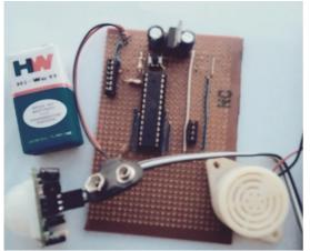
Figure 7: The Completed PIR Intrusion System Board
