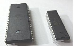
Figure 3: Atmega32 and Atmega8 Microcontroller. (Source: Microcontroller Wikipedia 2014)
