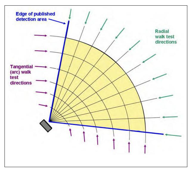
Figure 9: Recommended walk test paths and directions for the performance testing of a PIR sensor (Source: United States Nuclear Regulatory Commission
