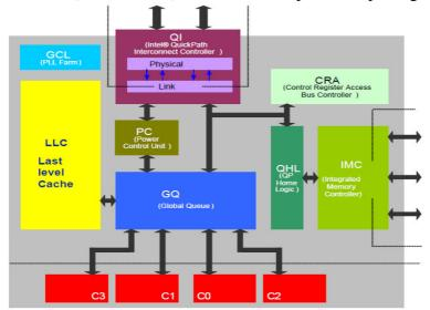
Figure 5 block diagram of the Intel® Xeon<sup>™</sup> 5500 processor
