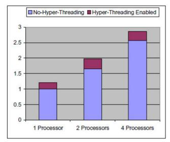
Figure 6: Performance increases HTT on an Online Transaction
