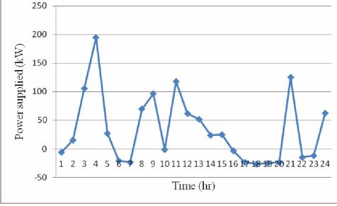
Figure 4: New power profile without diesel generator.
