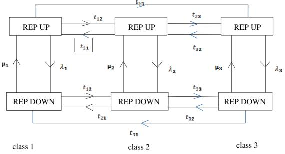
Figure 7: Proposed Markov model. where, REP is the renewable energy output power
