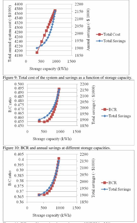
Figure 11: Effects of increasing the rated power of WECS by 25%.
