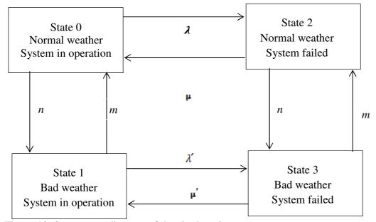
Figure 13: State space diagram of the single unit. The differential equation of the model is defined as
