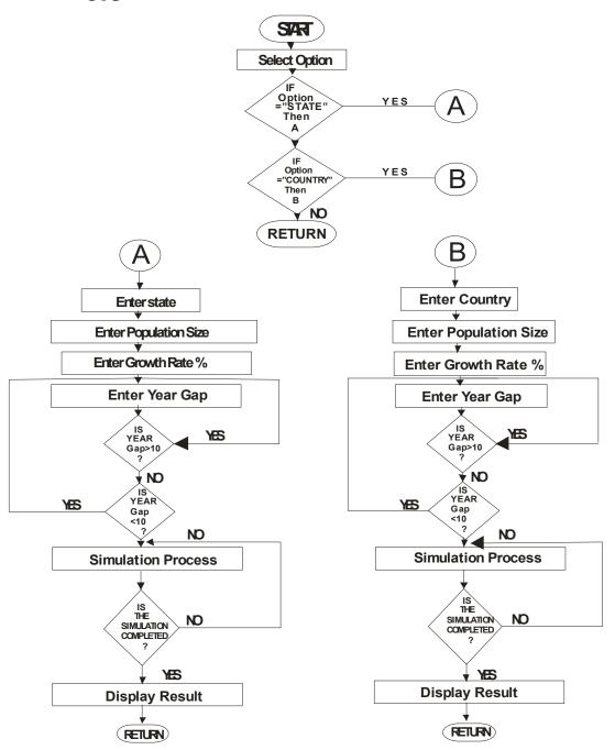
Fig.5: Program Flowcharts for operation procedure for the simulation model
