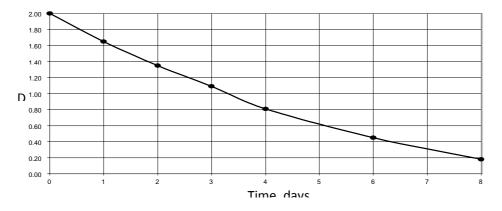
Figure. 11. The rate of deposition of suspended particles (D – optical density).
