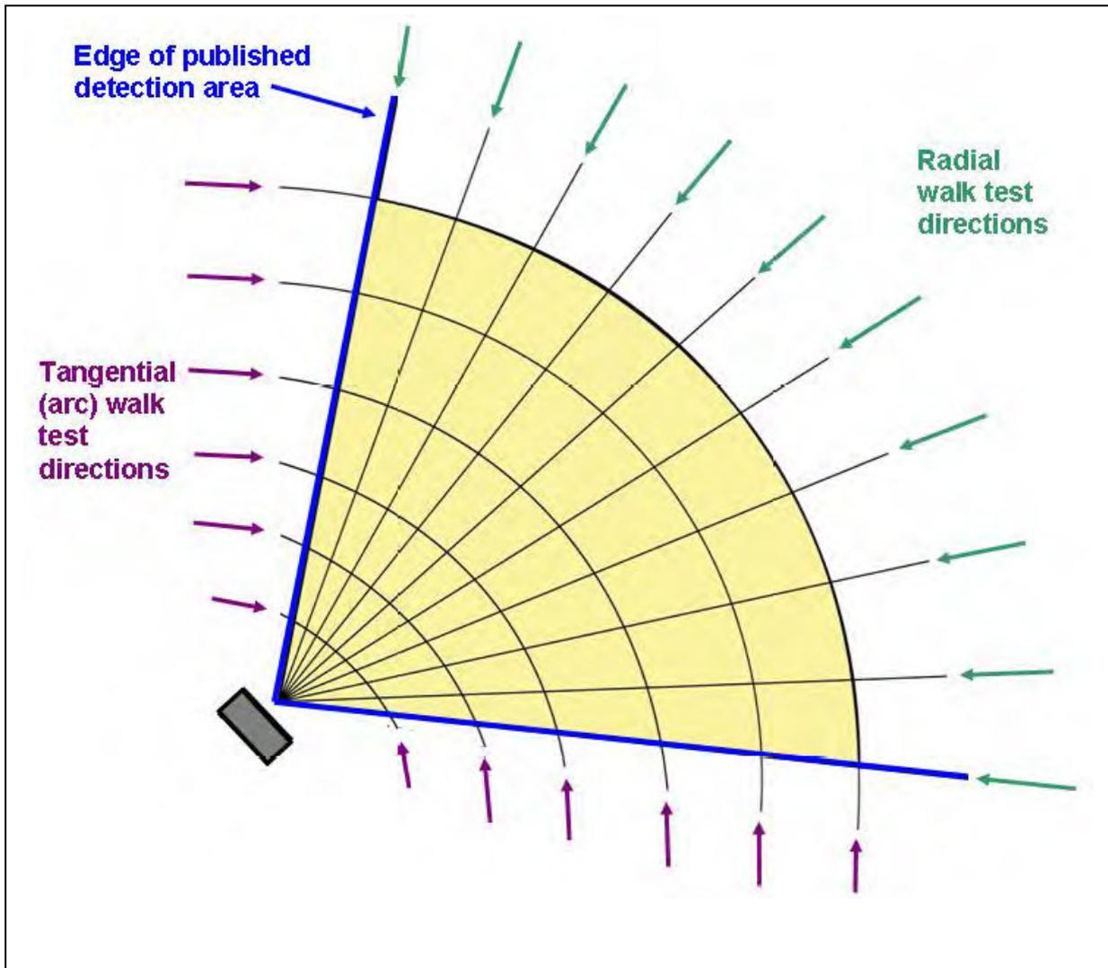
**Figure 9: Recommended walk test paths and directions for the performance testing of a PIR sensor (Source: United States Nuclear Regulatory Commission)**
