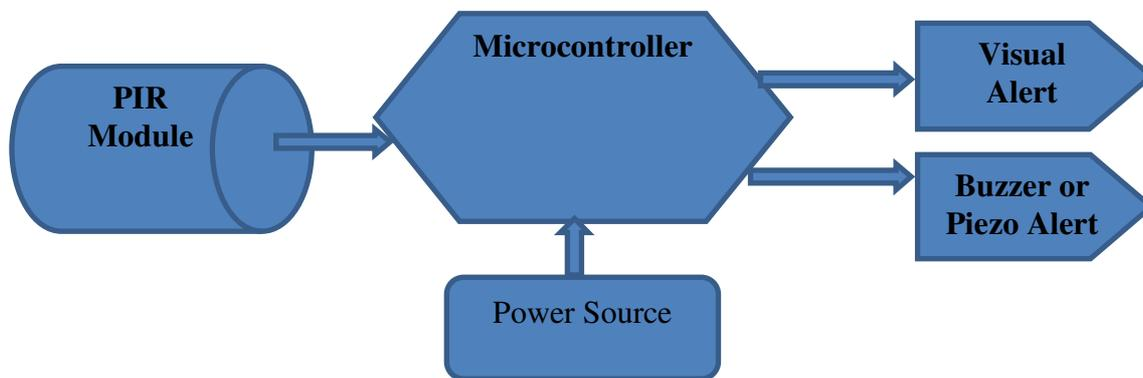
**Figure 1: Block Diagram Showing Design Modules and the Direction of Data Flow**
