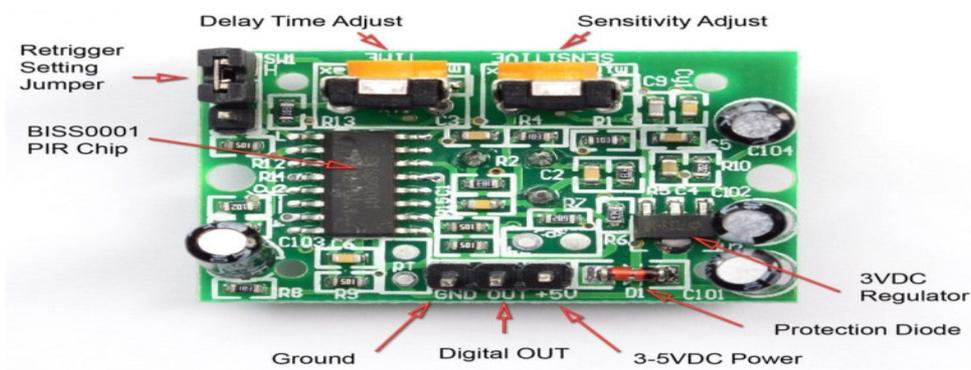
**Figure 2: PIR module's upper view. (Source: PIR Motion Sensor, Adafruit 2014)**
