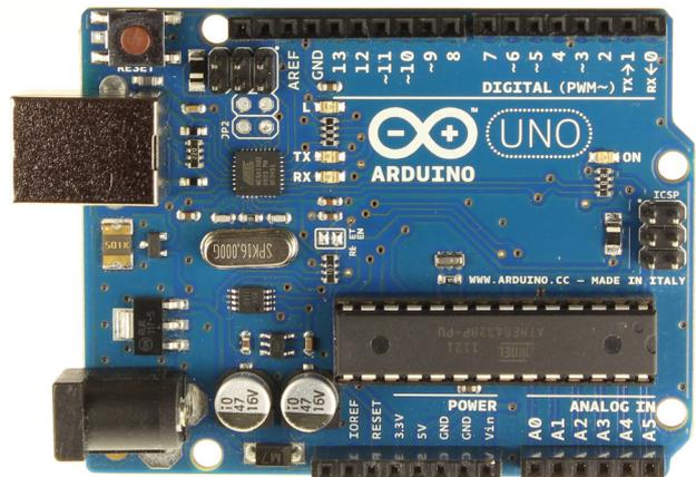
Figure 5: Most commonly used Arduino hardware platform. (Source: Arduino Boards)
