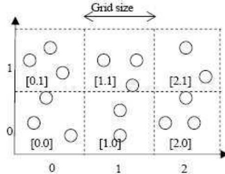
Fig.2. Grid Indexing
