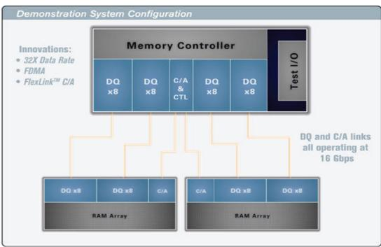
Fig. 2: The Rambus Terabyte Bandwidth Initiative
