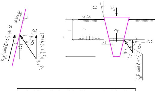
Fig. 6: Determination of Earth Pressure Coefficient K<sub>0</sub>
