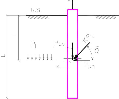
Fig. 7: Forces acting on a Rough Pile Shaft due to Uplift Load
