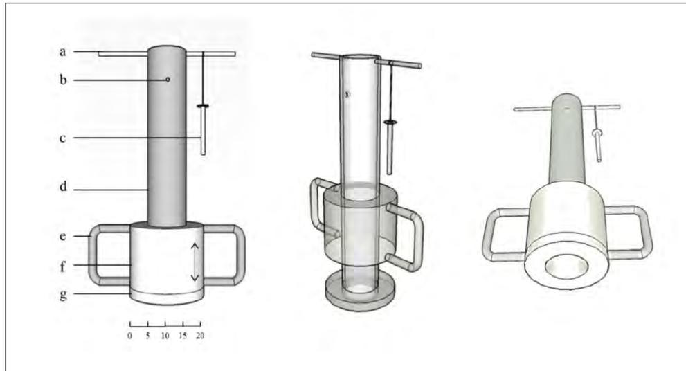
**Figure 1.** Scaled diagram of the hammer corer: a) top handle, b) hole in sleeve for core barrel securing pin, c) securing pin, d) stainless steel barrel which acts as the hammer slide, e) hammer handle, f) sliding hammer, and g) impact flange.
