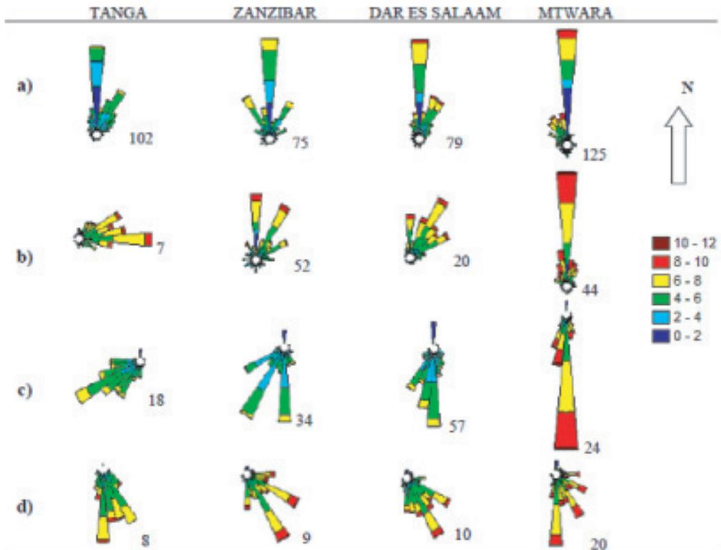
Figure 5. Wind rose diagrams plotted using Tanzanian coastal weather data for 1977-2006 in (a) January at 09:00, (b) January at 15:00, (c) July at 09:00 and (d) July at 15:00. The corresponding number of calms per month at each station is shown below the wind roses. The legend depicts wind speed in  $m.s^{-1}$ .
