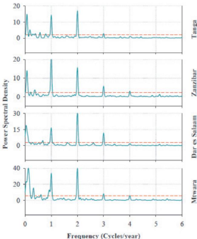
Figure 6. Spectral time series of monthly mean Tanzanian coastal wind velocities during 1977-2006. The red dashed line indicates the 95% Confidence Level.
