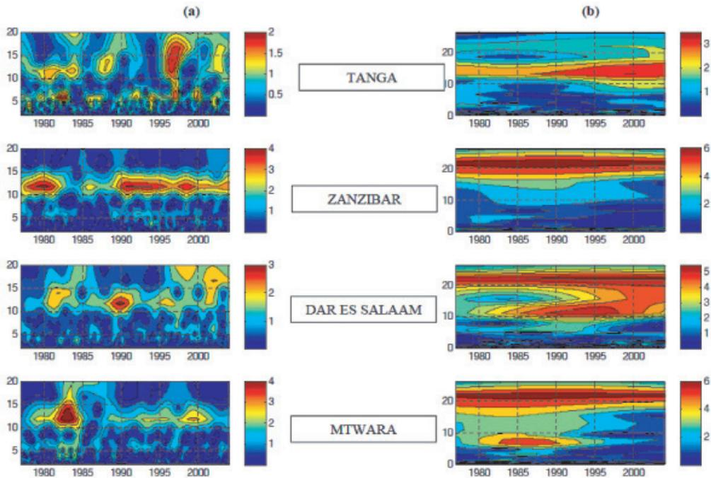
Figure 7. Morlet wavelet spectra representing (a) monthly maximum wind speeds and (b) low frequency oscillations in years along the Tanzanian coast. The legends indicate wind speed in  $\text{m.s}^{-1}$ .
