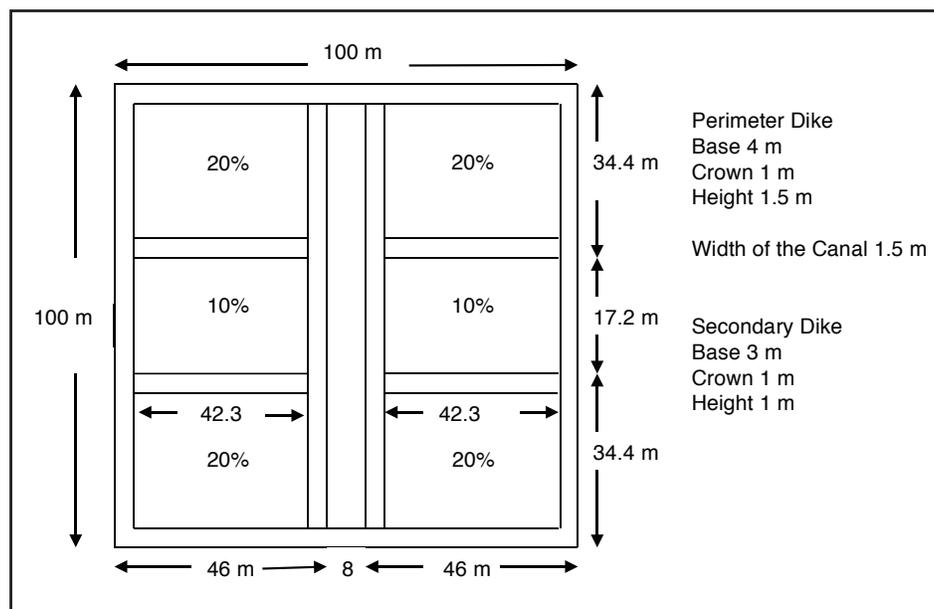
Fig. 1. Specification of the demonstration ponds constructed at Mtwara, Pemba and Tanga.
