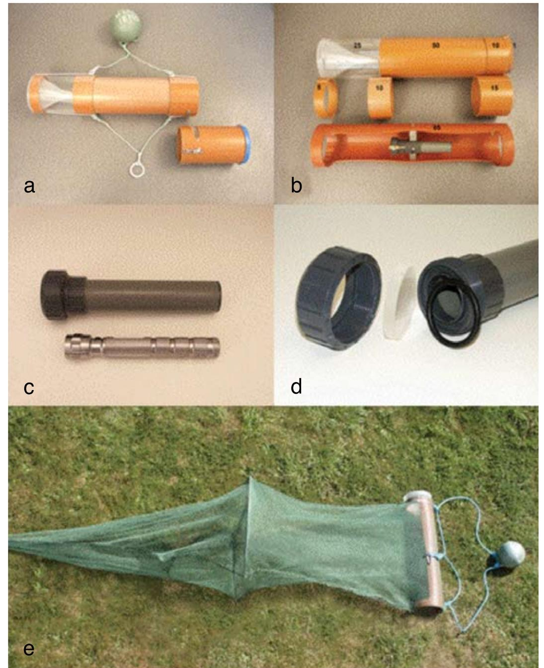
Plate 1. a) The IMR Standard Light Trap including an optional live animal collector. b) The different cut tube sections and a “fish and krill” version of the trap with the mounted torch. Numbers give the tube lengths in cm. c) The torch and its water proof tube casing. d) Details of the tube casing. e) The “fish and krill” version of the trap
