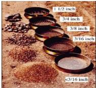
Figure 2: Standard sieve of sizes
