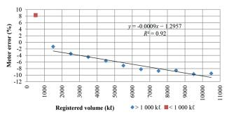
**Figure 7** Median meter error versus registered volume
