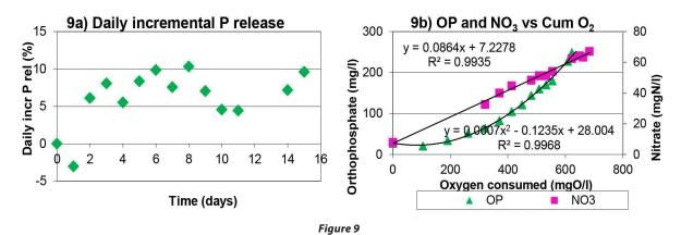
Polyphosphate release results of dilute batch test on NDBEPR WAS: (a) daily incremental P release expressed as a percentage and (b) orthophosphate and nitrate vs cumulative oxygen
