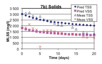
**Figure 7** Measured vs predicted (a) nitrate and (b) mixed liquor solids for dilute batch on NDBEPR WAS
