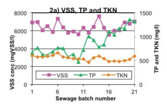
total phosphorus (TP) of about 1 200 mg P/ $\ell$  in a WAS of 6–7 g VSS/ $\ell$  during sewage batches 15 to 21.
