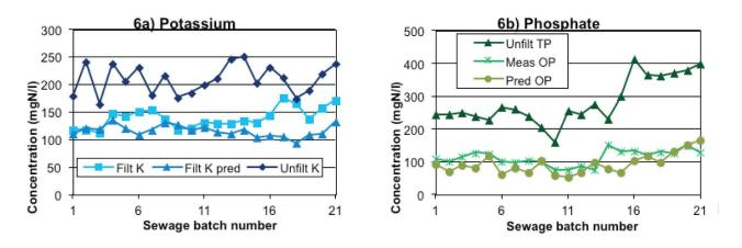
**Figure 6** Low-TSS digester's (a) potassium and (b) phosphate – filtered, unfiltered and predicted filtered (polyphosphate release at rate bG)
