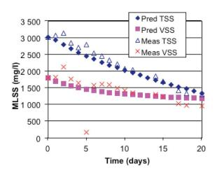
**Figure 10** Improved prediction of TSS on results of dilute batch test on NDBEPR WAS, using observed linear orthophosphate release
