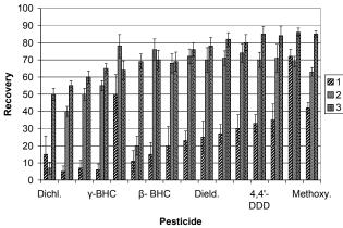
Figure 3 Recoveries of pesticides after SFE of a spiked sediment sample
