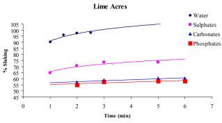
**Figure 6** The effect of sulphate, carbonate and phosphate ions on the hydration rate of Lime Acres lime
