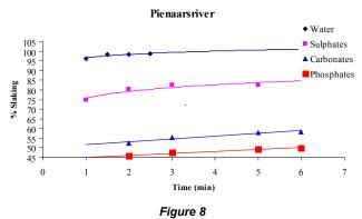
The effect of sulphate, carbonate and phosphate ions on the hydration rate of Pienaarsriver lime
