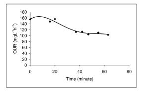
**Figure 6** OUR profile for Study B (F/M=0.17 mgCOD·mg<sup>-1</sup>VSS)
