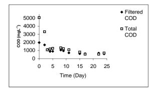
Figure 1 COD profile in reactor 1
