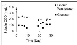
Figure 4 COD profiles of filtered wastewater and glucose reactor (Study C)
