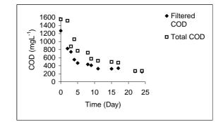
Figure 2 COD profile in reactor 2
