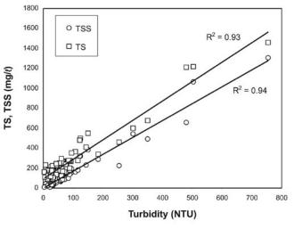
**Figure 2** Relationship between the turbidity measured in the laboratory and TS and TSS
