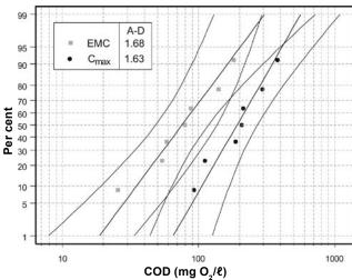
The analysis of the probability distribution has been carried out for TSS, TDS, TS and COD (Fig. 5) using the maximum concentration and the EMC. Acceptable fits were obtained with A-D values ranging between 1.31 and 1.68.
