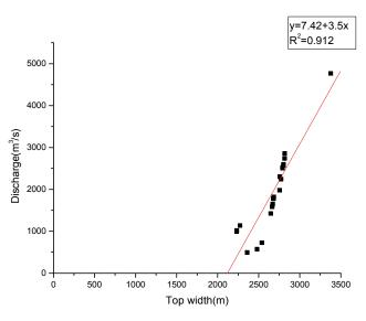
**Figure 3** Scatter plot: Discharge vs. top width
