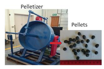
**Figure 1** Pelletization of waste gypsum in a disc pelletizer
