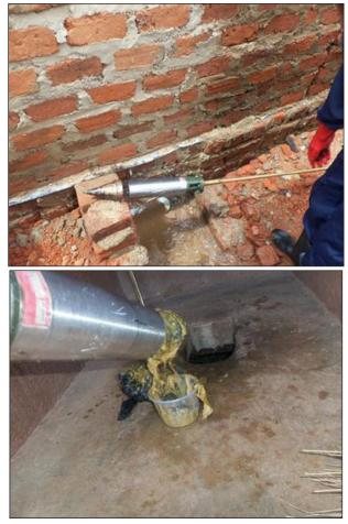
**Figure 3** Pit sludge sampler (Makerere University, 2015)
