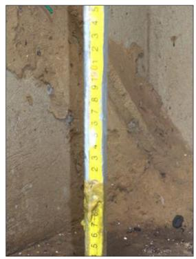
**Figure 4** Depth tool with sludge markings (Makerere University, 2015)
