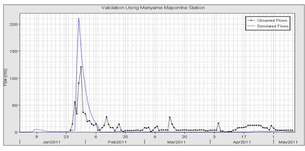
**Figure 5** Performance of the model when used on the Manyame Catchment
