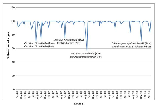
Percentage removal of algae at Vaalkop DWTW. Where <80% removal of algae occurred, the dominant algal genera in the raw water (indicated as 'Raw' on the graph) and potable water (indicated as 'Pot' on the graph) are displayed.
