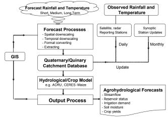
**Figure 1** A schematic flow chart demonstrating the structure of the agrohydrological forecasting framework
