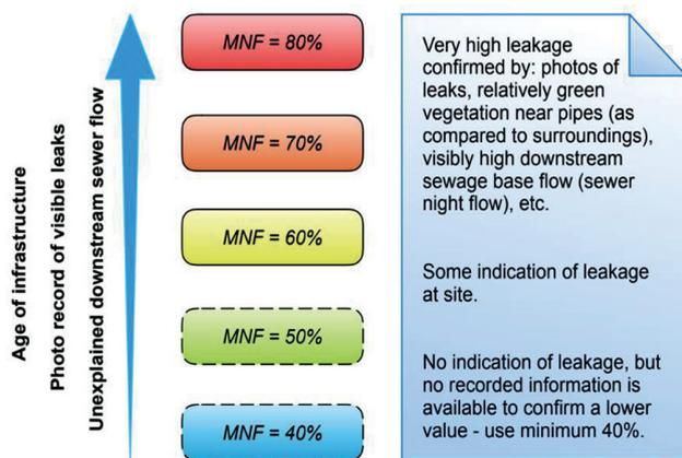
Figure 4. The record-based estimate of MNF (REM)
