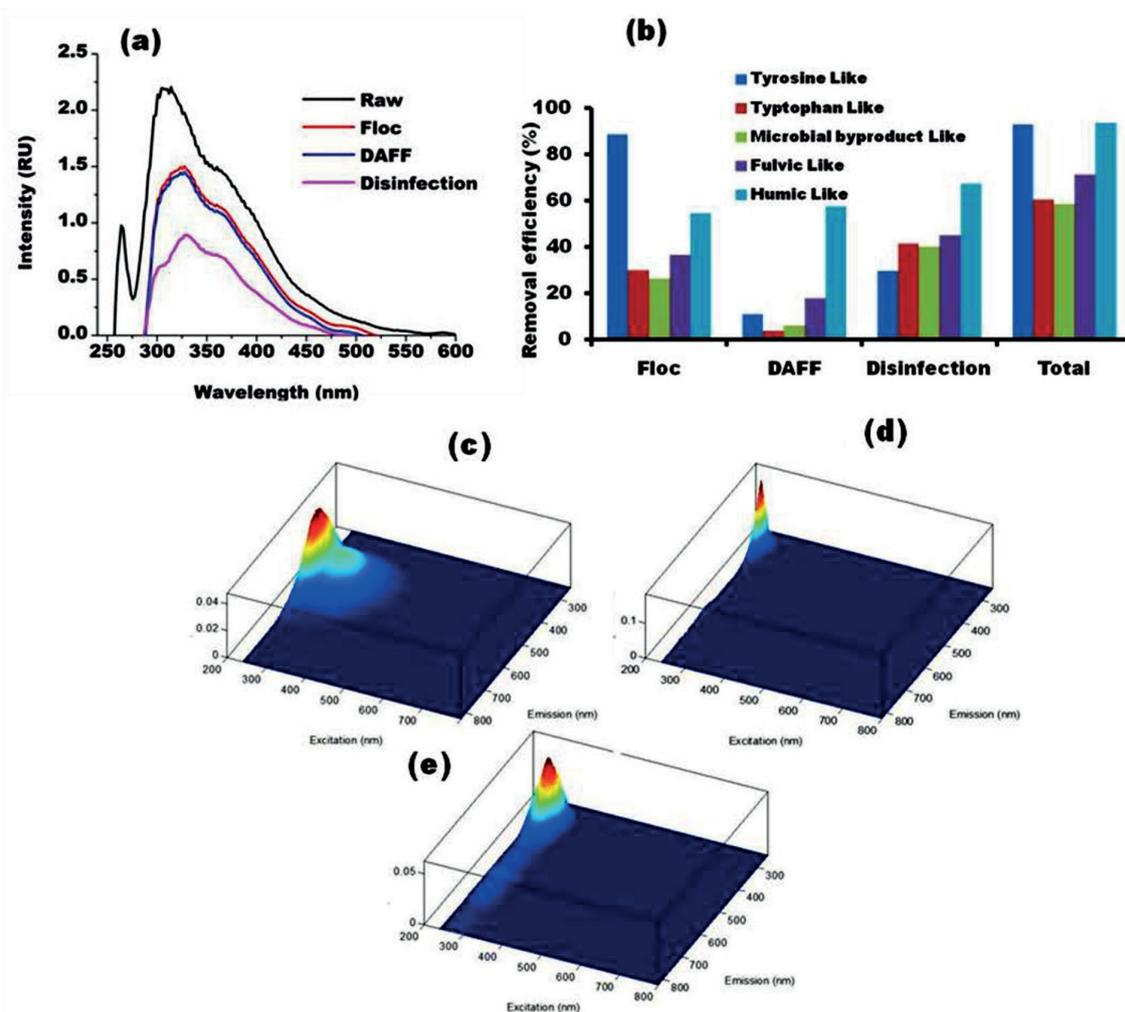
**Figure 5.** Fluorescence characteristics of water at different treatment stages (a) Synchronous scan of water samples after each treatment stage, (b) Removal efficiency of NOM fractions in the water samples after each treatment stage. Validated fluorescent components derived from the Parafac model on drinking water sources showing (c) Component 1 (C1), (d) Component 2 (C2) and (e) Component 3 (C3)
