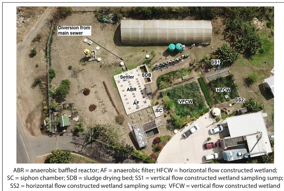
**Figure 1.** Aerial view of the Newlands Mashu demonstration-scale decentralised wastewater treatment system (DEWATS) within the eThekweni Municipality (taken September 2019)
