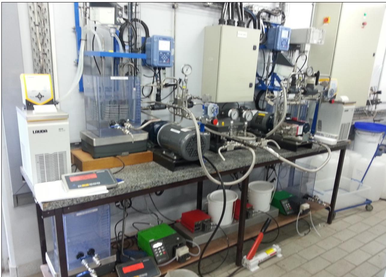
**Figure 2.** Photograph of a forward osmosis experimental set-up
