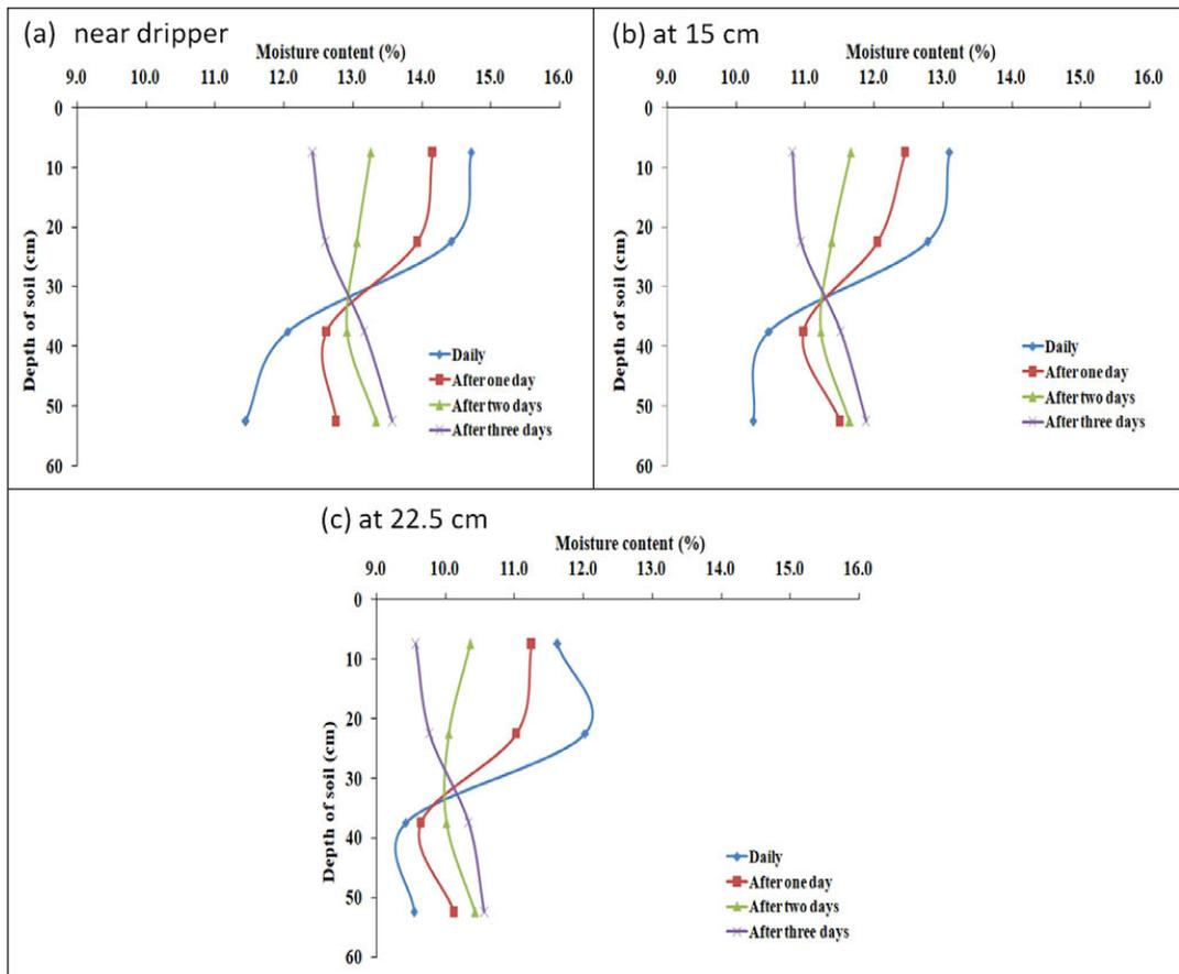
**Figure 7.** Radial and vertical movement of moisture in the root zone at 60 DAS at 60 cm lateral spacing: (a) near dripper, (b) at 15 cm, and (c) at 22.50 cm
