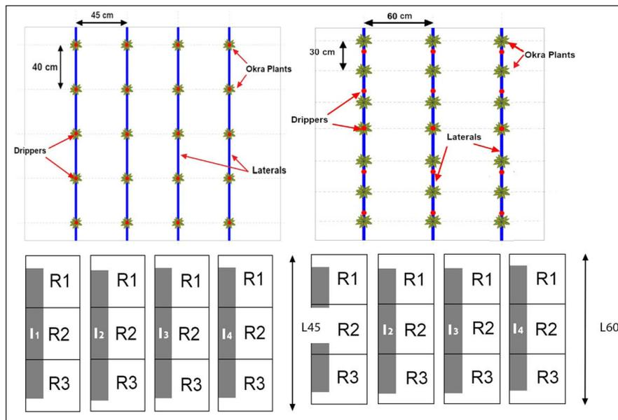
**Figure 2.** Layout of the experiment with 45 and 60 cm lateral spacing used in the study area
