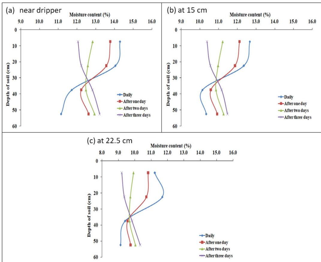
**Figure 8.** Radial and vertical movement of moisture in the root zone at 90 DAS at 60 cm lateral spacing (a) near dripper, (b) at 15 cm, and (c) at 22.50 cm
