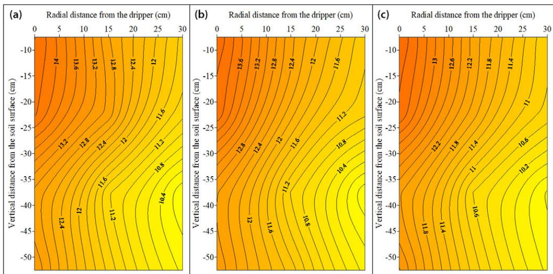
**Figure 14.** Moisture content contour map at alternate day irrigation frequency under (a) 30, (b) 60 and (c) 90 DAS at 60 cm lateral spacing
