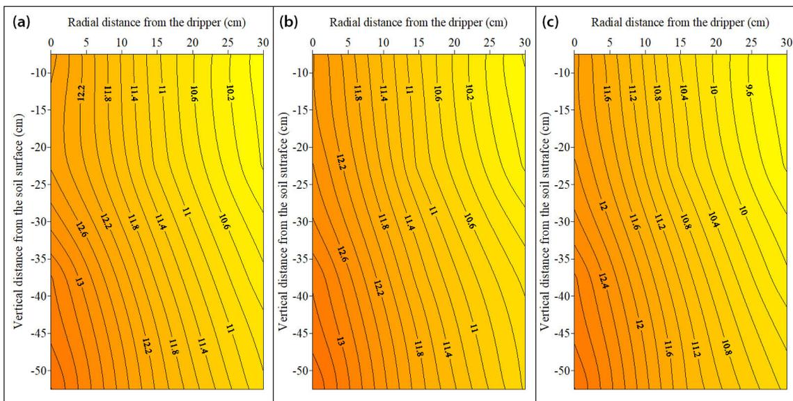
**Figure 16.** Moisture content contour map with after-3-day irrigation frequency under (a) 30, (b) 60 and (c) 90 DAS at 60 cm lateral spacing
