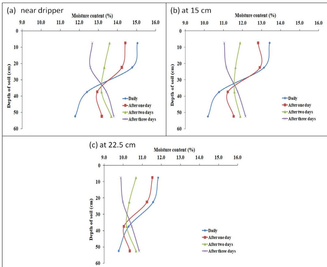
**Figure 6.** Radial and vertical movement of moisture in the root zone at 30 DAS at 60 cm lateral spacing: (a) near dripper, (b) at 15 cm, and (c) at 22.50 cm
