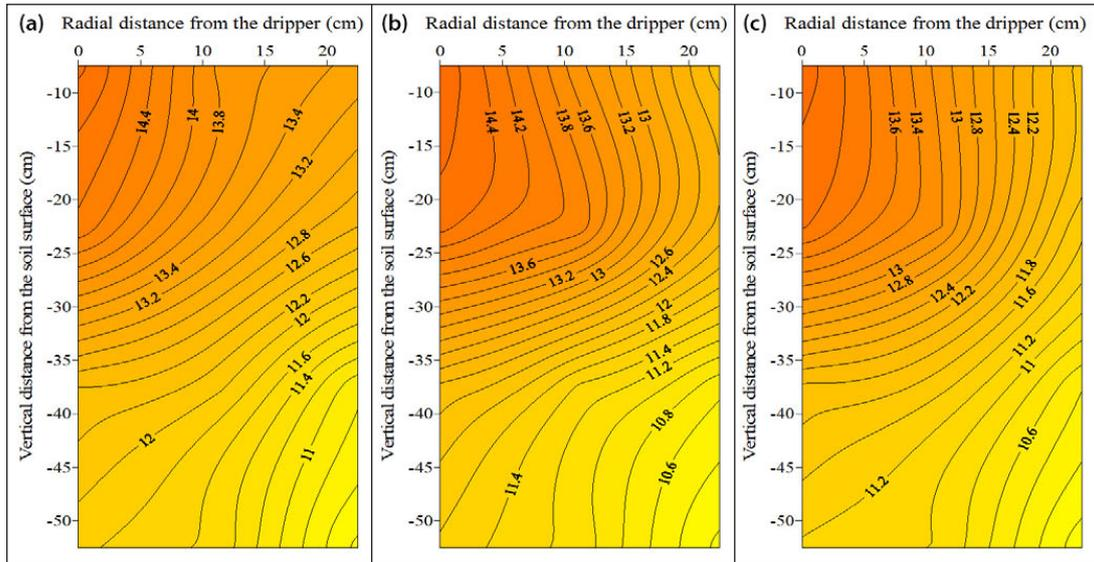
**Figure 9.** Moisture content contour map at daily irrigation frequency under (a) 30, (b) 60 and (c) 90 DAS at 45 cm lateral spacing
