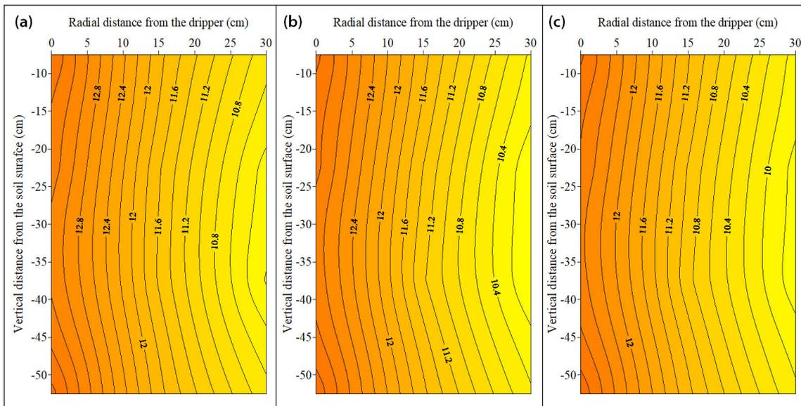
**Figure 15.** Moisture content contour map with after-2-day irrigation frequency under (a) 30, (b) 60 and (c) 90 DAS at 60 cm lateral spacing
