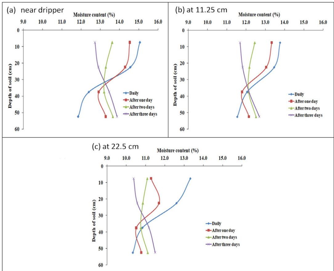
**Figure 3.** Radial and vertical movement of moisture in the root zone at 30 DAS at 45 cm lateral spacing: (a) near dripper, (b) at 11.25 cm, and (c) at 22.50 cm
