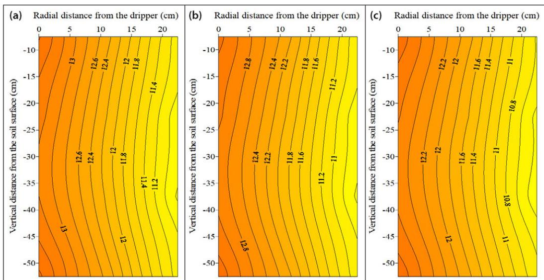
**Figure 11.** Moisture content contour map with after-2-day irrigation frequency under (a) 30, (b) 60 and (c) 90 DAS at 45 cm lateral spacing
