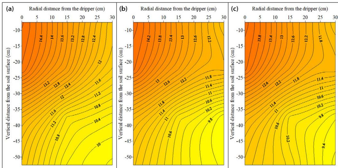
**Figure 13.** Moisture content contour map at daily irrigation frequency under (a) 30, (b) 60 and (c) 90 DAS at 60 cm lateral spacing
