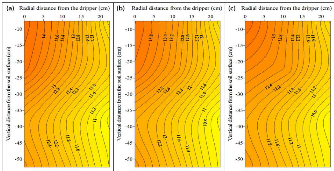
**Figure 10.** Moisture content contour map at alternate day irrigation frequency under (a) 30, (b) 60 and (c) 90 DAS at 45 cm lateral spacing
