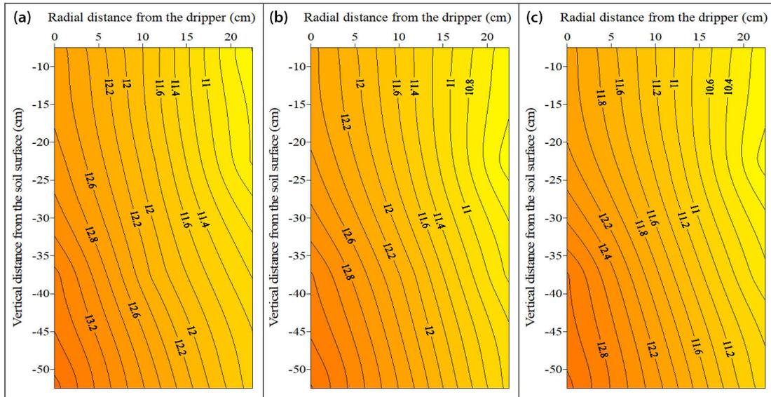
**Figure 12.** Moisture content contour map with after-3-day irrigation frequency under (a) 30, (b) 60 and (c) 90 DAS at 45 cm lateral spacing
