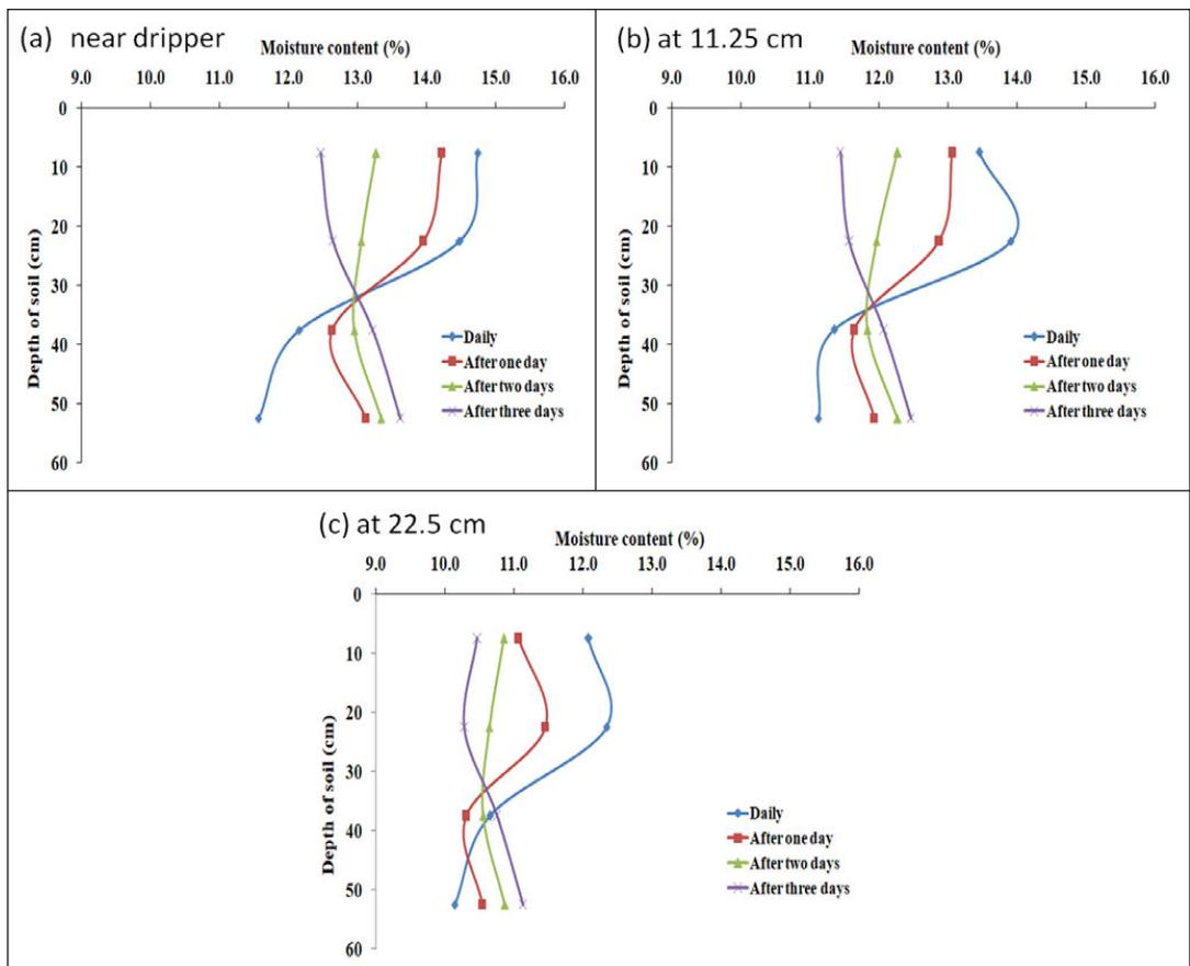
**Figure 4.** Radial and vertical movement of moisture in the root zone at 60 DAS at 45 cm lateral spacing: (a) near dripper, (b) at 11.25 cm, and (c) at 22.50 cm
