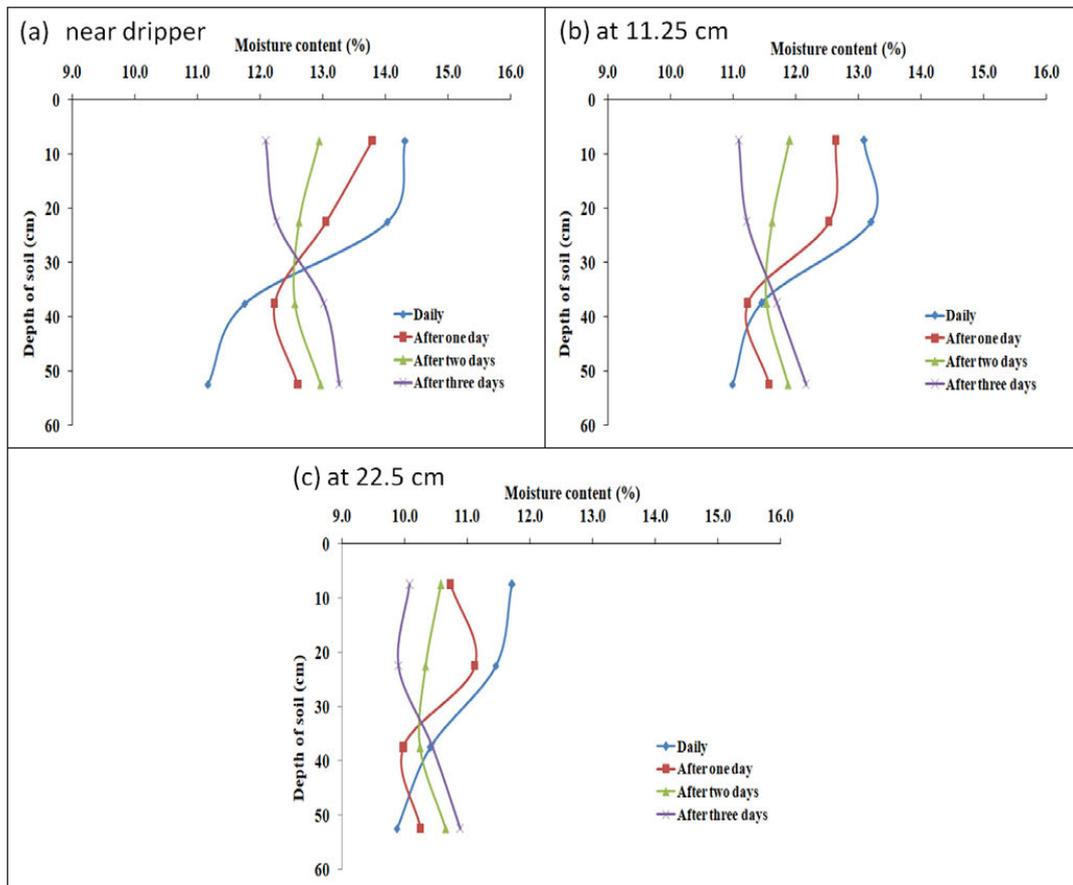
**Figure 5.** Radial and vertical movement of moisture in the root zone at 90 DAS at 45 cm lateral spacing: (a) near dripper, (b) at 11.25 cm, and (c) at 22.50 cm
