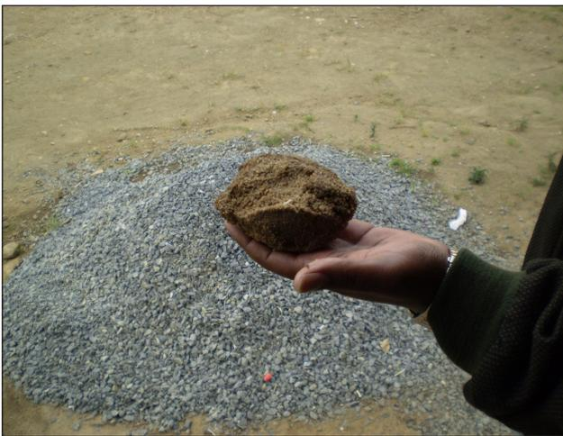
**Figure 9.** Mudball resulting from the use of organic coagulant
