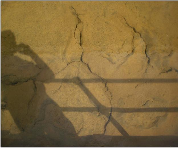
**Figure 7.** The effect of organic coagulant–formed suspension on filtration – the ruptures passing into filter media result from filter operation under sub-atmospheric pressure conditions
