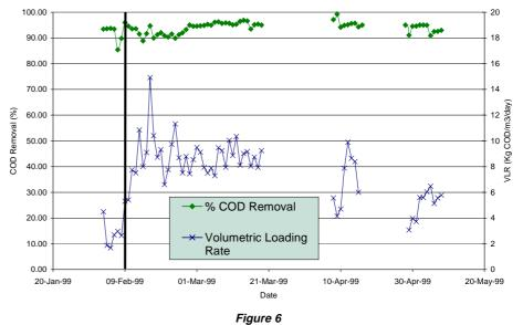
Percentage COD removal efficiency vs. volumetric loading rates for 1999
