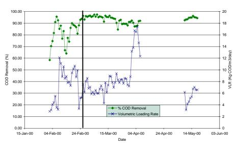
Figure 7 Percentage COD removal efficiency vs. volumetric loading rates for 2000
