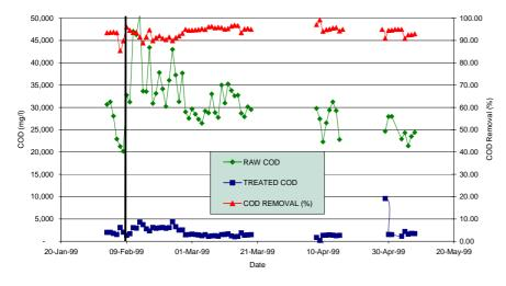
**Figure 3** Raw and treated COD values with COD removal efficiency for 1999
