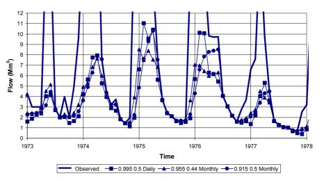
Figure 6 Observed flows and separated baseflows for gauge W5H005
