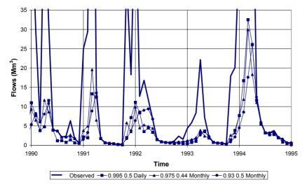
**Figure 3** Observed flows and separated baseflows for gauge T3H002
