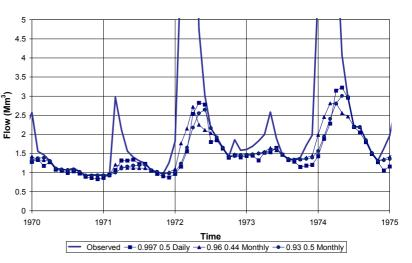
Figure 1 Observed flows and separated baseflows for gauge X3H003
