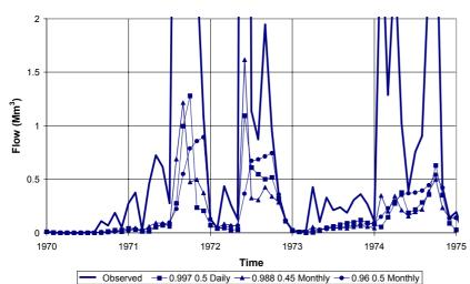
**Figure 4** Observed flows and separated baseflows for gauge J3H012
