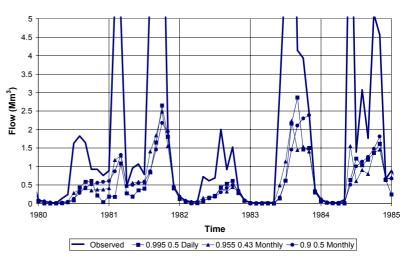
Figure 2 Observed flows and separated baseflows for gauge G4H014
