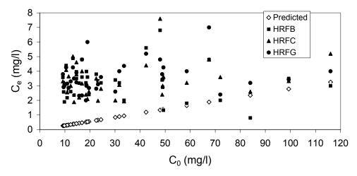
Figure 2 Comparison of observed Ce versus predicted Ce for the HRF units
