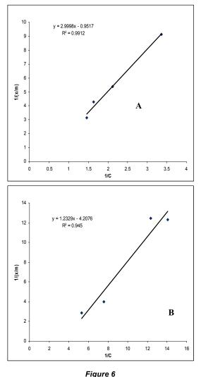
Langmuir isotherms for biosorption of (A) Cu(II) and (B) Co(II)
