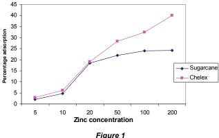
Percentage adsorption of Zinc by adsorbents at different concentrations
