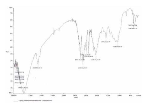
Figure 4 Infrared spectrum of sugarcane biomass
