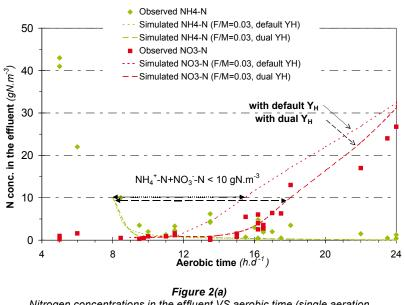
Nitrogen concentrations in the effluent VS aerobic time (single aeration tank, 10°C) - Observed vs. simulated values (Run 1, F/M = 0.03 kg BOD<sub>c</sub> (kg MLVSS d)<sup>-1</sup>)
