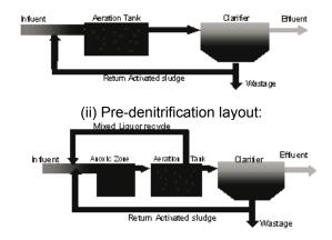
**Figure 1** Virtual layouts (single aeration tank and pre-denitrification layouts) used to perform the simulations
