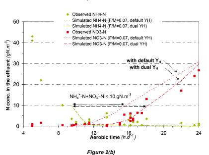
Nitrogen concentrations in the effluent VS aerobic time (single aeration
