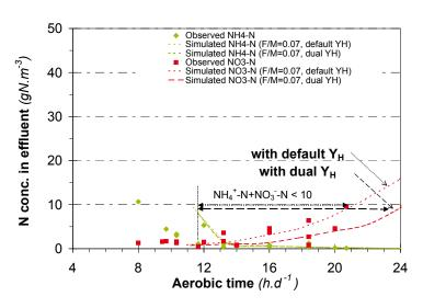
Figure 3(b) Nitrogen concentrations in the effluent vs. aerobic time (pre-denitrification layout, 10°C) - Observed vs. simulated values (Run 2, F/M = 0.07 kg BOD<sub>s</sub>·(kg MLVSS·d)<sup>-1</sup>)
