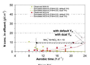
Figure 3(a) Nitrogen concentrations in the effluent vs. aerobic time (pre-denitrification layout, 10°C) - Observed vs. simulated values (Run 1, F/M = 0.03 kg BOD<sub>5</sub>·(kg MLVSS·d)<sup>-1</sup>)
