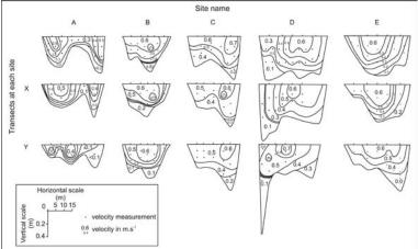
fastest average flows, with a velocity of greater than  $0.5~\text{m}^2\cdot\text{s}^{-1}$  at each (Fig. 6).
