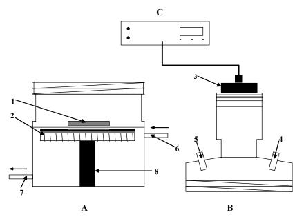
Figure 1 The PO<sub>2</sub> measuring cell (50 mℓ capacity), made from Perspex, to measure start and end PO<sub>2</sub> values. A, Perspex chamber; B, Perspex-head housing the Radiometer oxygen elektrode; C, Oxygen meter; The B part of the cell is screwed on part A. 1, magnetic stirrer; 2, water turbine; 3, Clark-polarographic oxygen electrode (Radiometer); 4, inlet for water sample; 5, outlet for water sample; 6, water inlet and, 7, water outlet for turbine; 8, axle. Scale, 1 : 1 cm.
