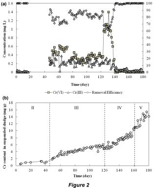
(a) Effluent Cr(III) and Cr(VI) concentrations and Cr(VI) removal efficiency and (b) total Cr concentration in the sludge during the operational period
