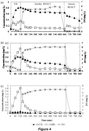
Concentration profiles of Cr(III), Cr(VI) and DO in SBR during the FILL and REACT periods in phases (a) III, (b) IV and (c) V
