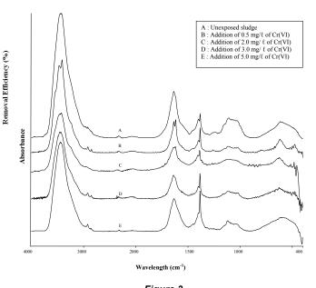
Figure 3 FTIR spectra of activated sludge before and after Cr(VI) addition
