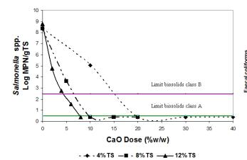
Figure 2 Removal of faecal coliforms in treated sludge with different CaO doses at different TS concentrations
