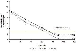
**Figure 4** Removal of faecal coliforms in treated sludge with different contact times at different concentrations of TS
