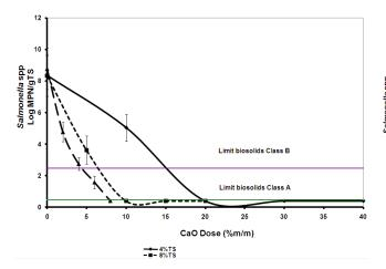
**Figure 3** Removal of Salmonella spp. in treated sludge with different CaO doses at different TS concentrations
