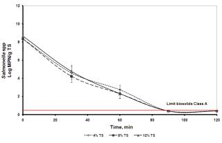
Figure 5 Removal of Salmonella ssp. in treated sludge with different contact times at different TS concentrations
