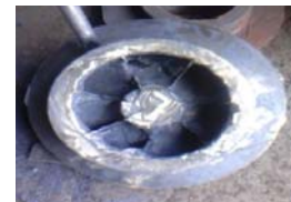
d. After outer grinding both surfaces
