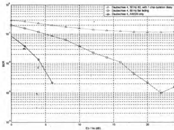
Figure 11 BER vs.  $E_b/N_o$  in AWGN, flat and ISI channel
