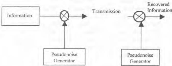
Figure 5 Block Diagram of a DS system
