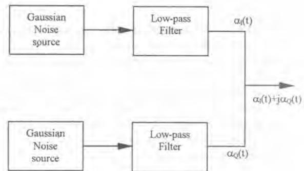
Figure 1 Fading simulator that uses low-pass filtered white Gaussian noise
