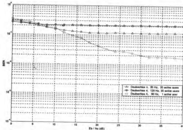
Figure 10 BER vs.  $E_b/N_o$  in ISI channel. The excess delay of the channel is assumed to be of one chip duration.
