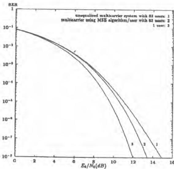
Figure 8 Performance on AWGN channel using DFT realization [8]
