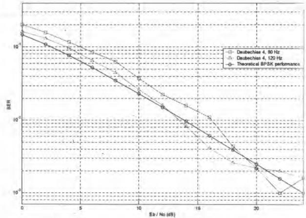
Figure 9 BER vs.  $E_b/N_0$  in flat fading channel
