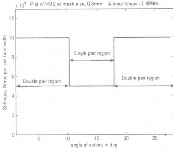
Figure 7 Simulation results of variable stiffness due to variation of contacting pairs
