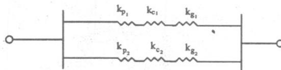
Figure 5 Springs connected in series and parallel.
