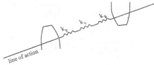
Figure 4 Mesh stiffness along line of action.
