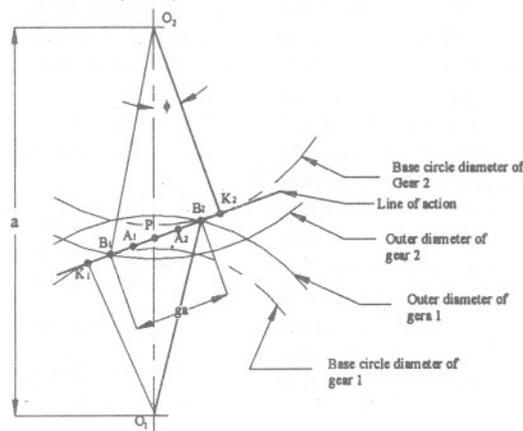
Figure 2 Meshing cycle along the line of action
