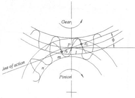
Figure 3 Position of mesh pair teeth
